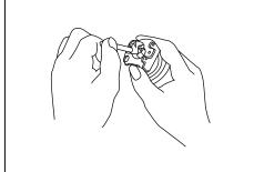
Install spindle over bar, rotate slightly and push into place. Slot on spindle should be on same side as slide jaws.
